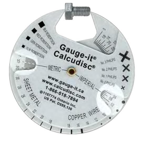
Using the calipers on your *Calcudisc*™, you can measure objects or areas up to 1.5″ long in both metric and imperial at the same time. As you will see by looking at the highlighted areas above, the bolt being measured is 15mm or 5/8″ long, both determined at the same time.
